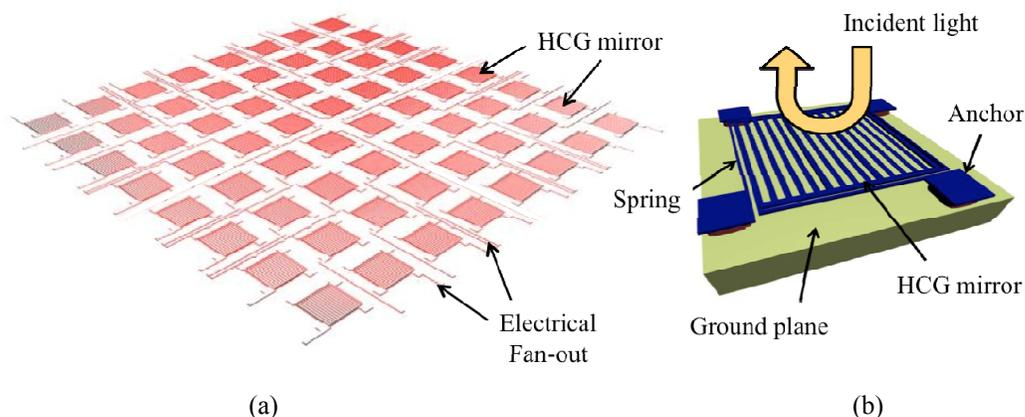
Figure 1. (a) Layout of the  $8 \times 8$  HCG array. (b) Schematic of the HCG mirror pixel.
