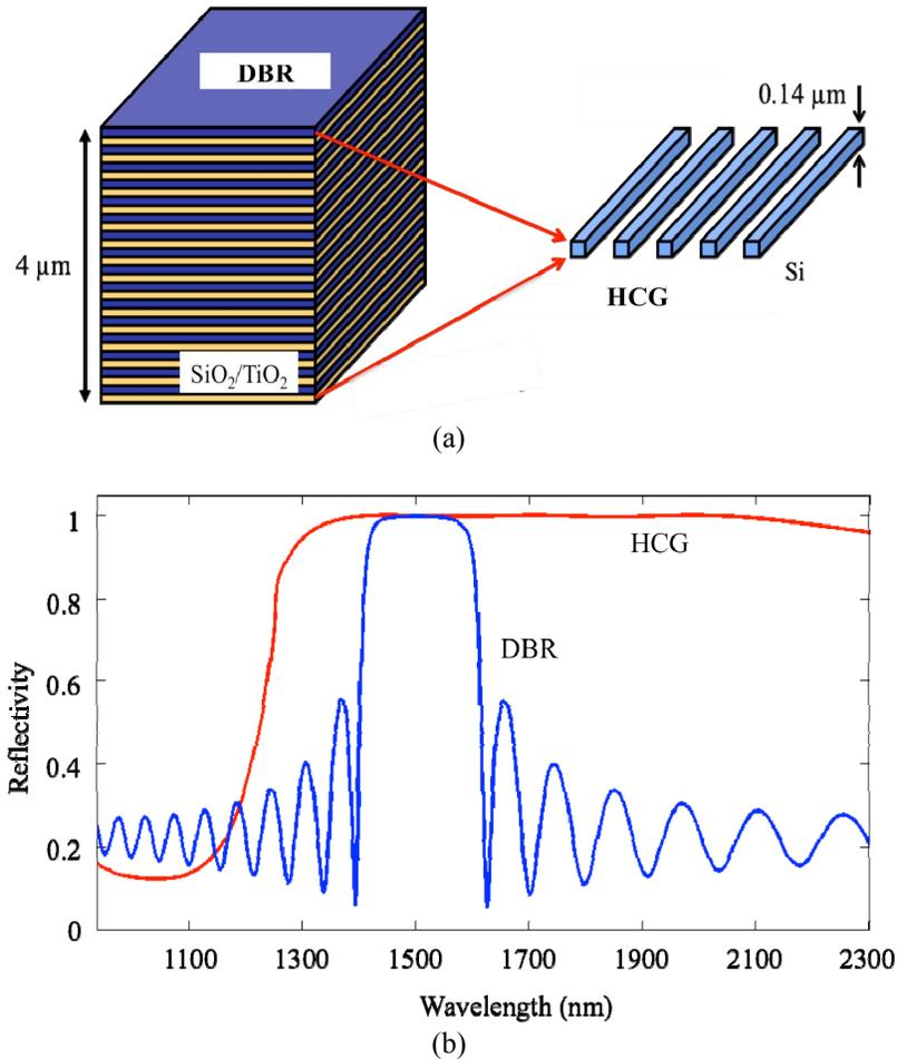
Figure 2. Lightweight HCGs show very high reflectivity along a broad bandwidth, wider than distributed Bragg reflectors (DBR). (a) HCG is lighter than DBR by 85 times for the same reflectivity of 99.5%. (b) HCG is highly reflective at the broad wavelength range compared to DBR.
