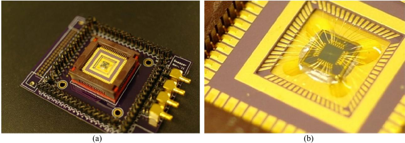
Figure 5. (a) Optical micrograph of the MEMS optical phased array mounted on a chip carrier, chip socket, and circuit board. (b) Close-up view of the packaged die with 64 gold wirebonds.
