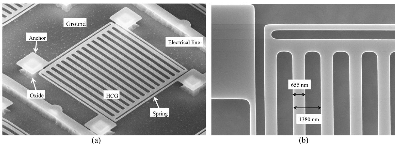
Figure 4. SEM images of the fabricated HCG mirror. (a) Released HCG mirror supported by four springs and anchors. (b) Fabricated HCG bars with period and width of 1380 nm and 655 nm, respectively.
