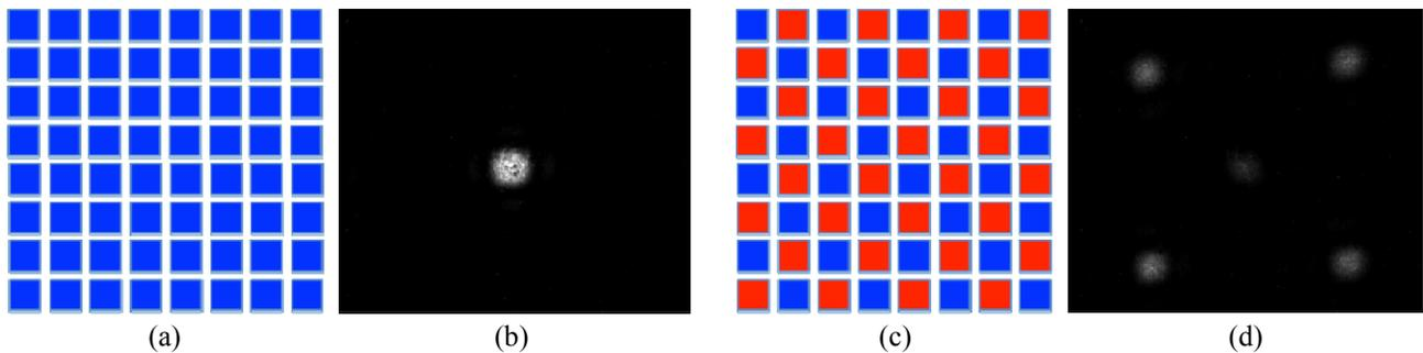
Figure 6. Beamsteering measurement results. (a) Phase map of unbiased phased array (blue: zero phase shift) and (b) the corresponding beamsteering pattern. (c) Phase map of binary checkerboard pattern (blue: zero phase shift, red:  $\pi$  phase shift) and (d) the corresponding far-field.
