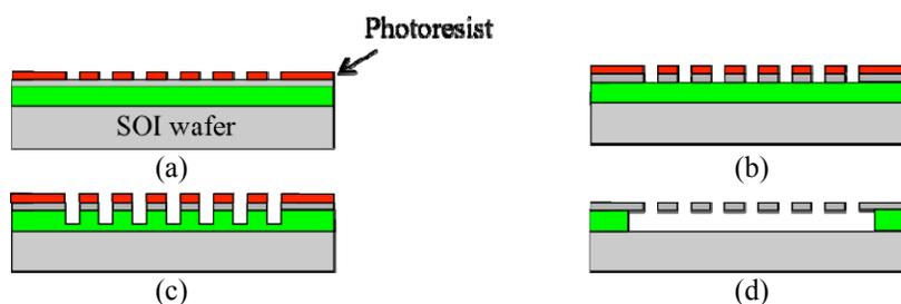
Figure 3. The fabrication process for HCG optical phased array. Only one photomask is needed. (a) Lithographic step using deep ultraviolet (DUV) stepper. (b) Dry etching of SCS HCG mirrors. (c) Partial dry etching of buried oxide layer to facilitate release etching. (d) Release of HCG mirrors using vaporized hydrofluoric (HF) acid.
